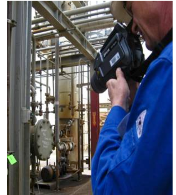
EPA inspector using an infrared camera to detect invisible organic chemical emissions. Photo: EPA
