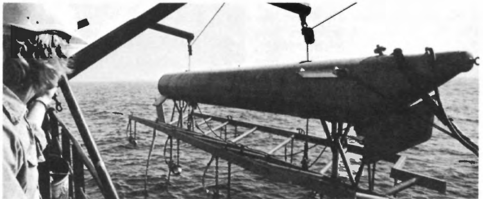
An air "gun" suspended from a float, is lowered from the stern of a Shell Oil Co. vessel. Pressure waves from the guns are directed downward through the water into rock layers below.
