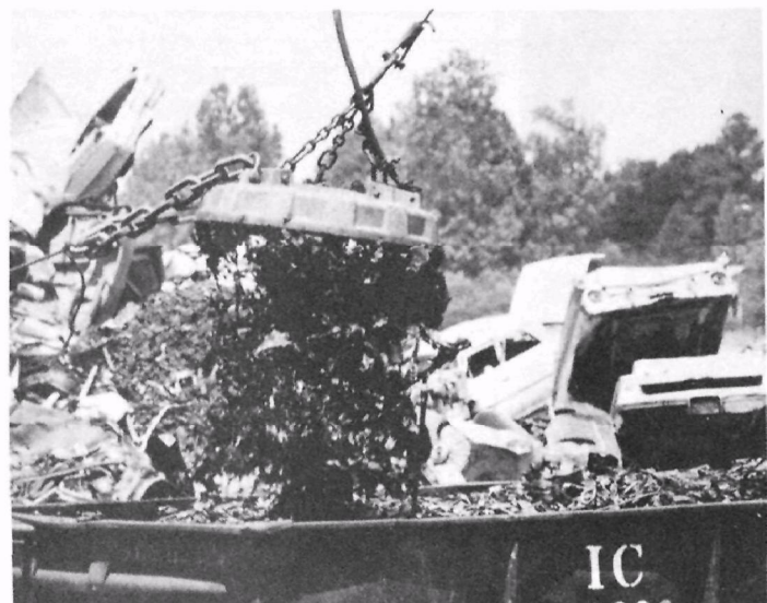
Shredded scrap is loaded by electromagnet crane for rail haul to the steel mill.
