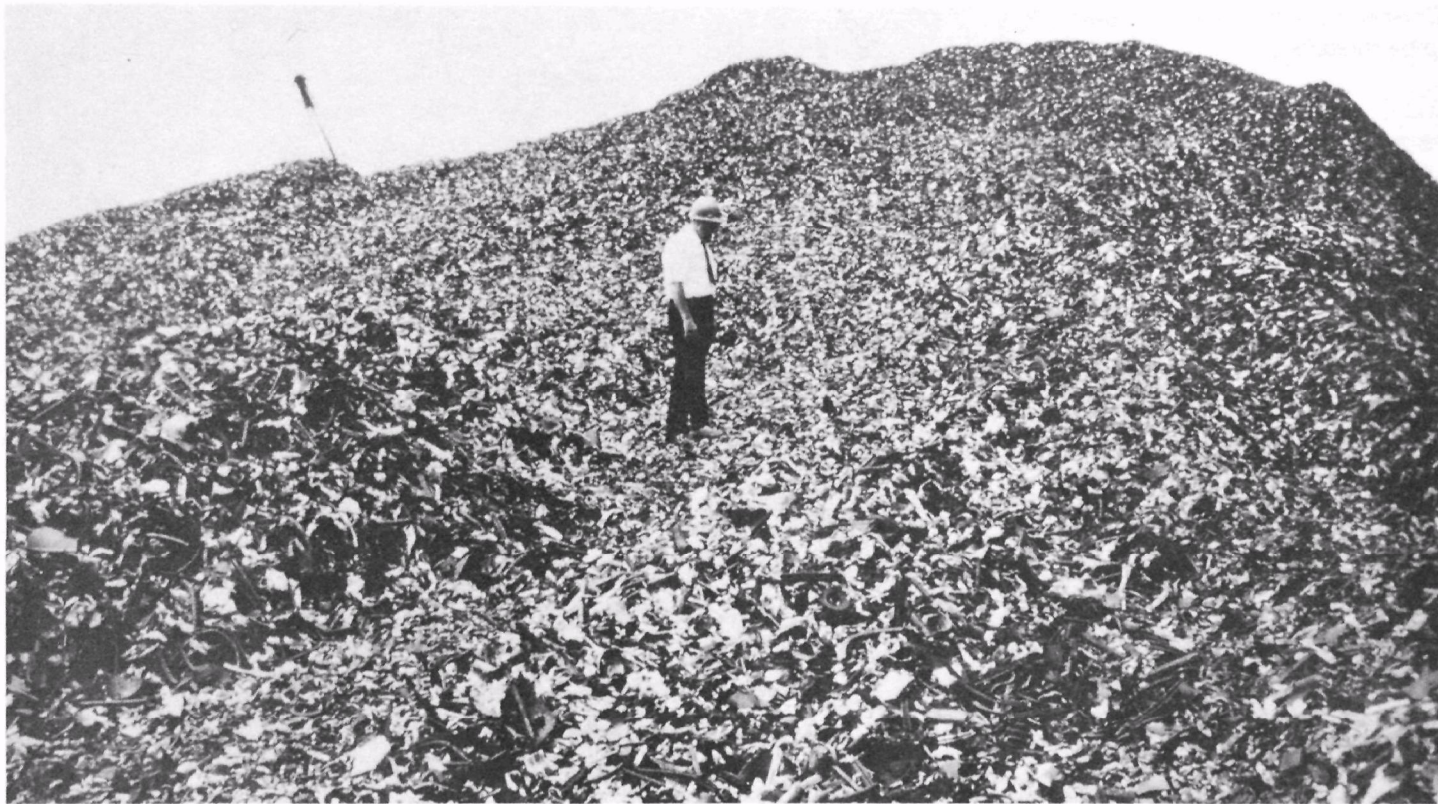
This mountain of steel fragments is the remains of 30,000 old automobiles which have been processed for remelting by steel mills and foundries.
