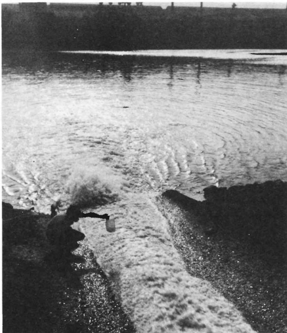
Permits to discharge waste water into rivers must be monitored regularly to insure compliance. Here a Pennsylvania State employee samples the water from an industrial outfall on the Monongahela River at West Mifflin, near Pittsburgh.
