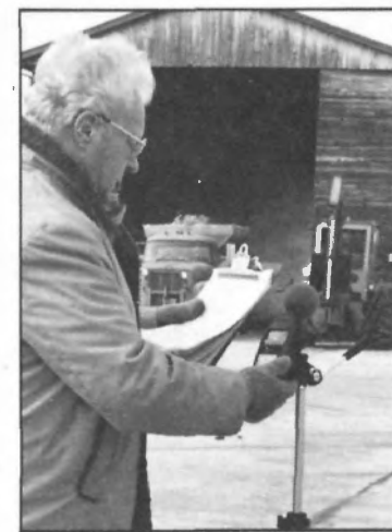
Vincent Flynn adjusts a sound meter to take noise measurements for use in developing a community-wide noise control program.
