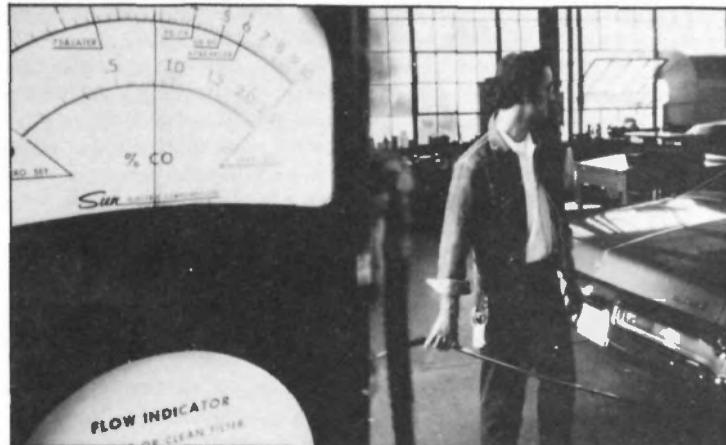
An employee of an auto emission inspection station in downtown Cincinnati holds hose which runs from the tailpipe to a machine which registers carbon monoxide and hydrocarbon emissions.
