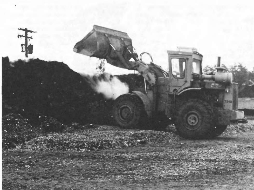
Steam rises from a composting sludge pile that is being mechanically mixed with wood
