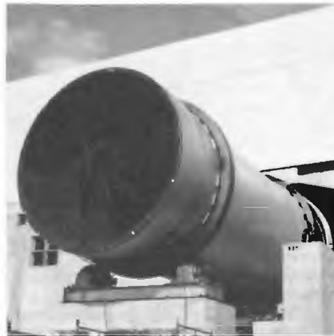
Incinerator designed to burn hazardous wastes at the 3M company near St. Paul, Minn.
