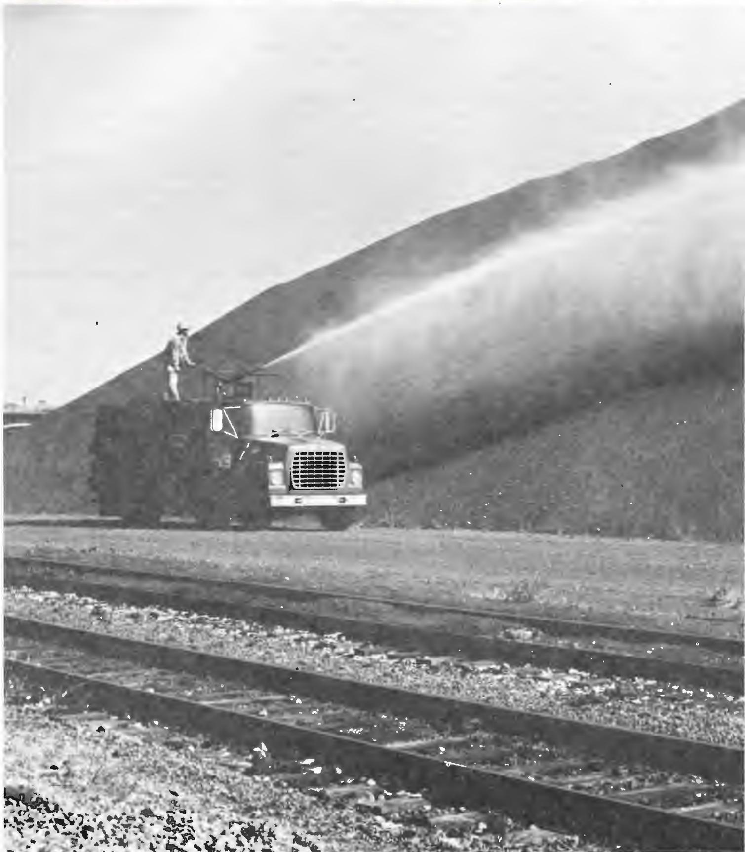
*Piles of iron ore pallets at Armco Steel's Middletown Works are sprayed to reduce dust.*
