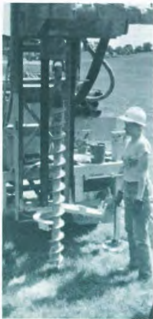
In a field hydrology class at Ohio's Wright State University, an instructor explains use of a rig to drill a ground-water monitoring well.
