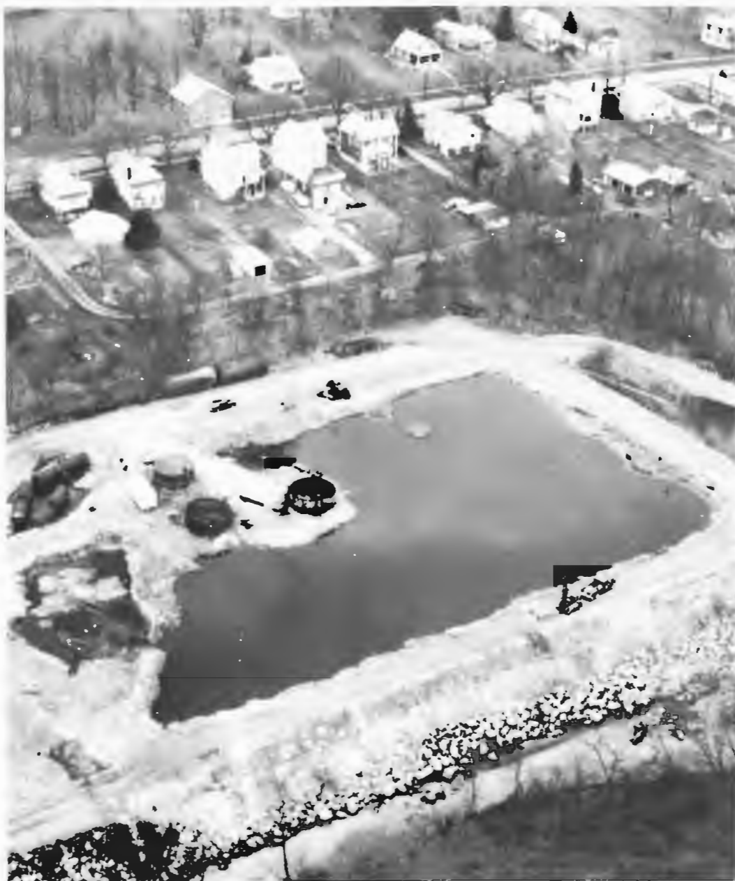
Bruin Lagoon, an abandoned hazardous waste site in Pennsylvania, next to a residential area. Wastes in the lagoon and storage tanks contaminated surface and ground water. The site is on EPA's National Priority List for Superfund action.
