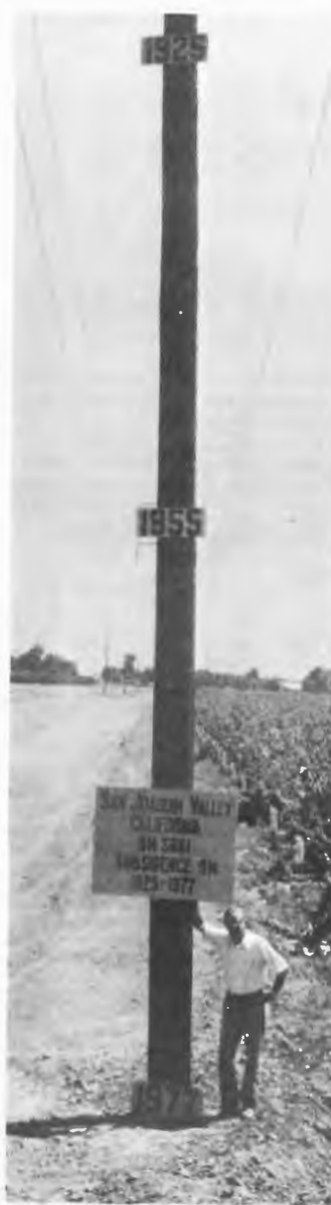
In certain areas of the country, ground-water quantity as well as quality can be a serious problem. Markers on this pole in California's San Joaquin Valley indicate a dramatic drop in the land surface — a loss of 29 feet between 1925 and 1977. The subsidence was caused by ground-water withdrawal, primarily for irrigation.
