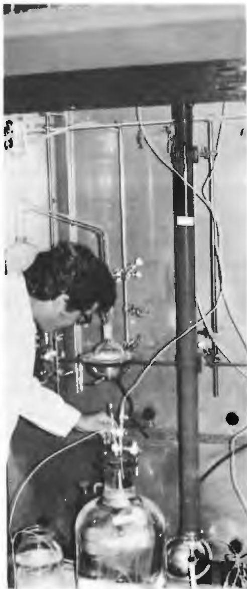
Work carried out at the EPA lab in Ada, Oklahoma is part of the agency's ground-water research program. Here a scientist determines biodegradation by passing water containing organic chemicals through columns of authentic, uncontaminated aquifer materials.
