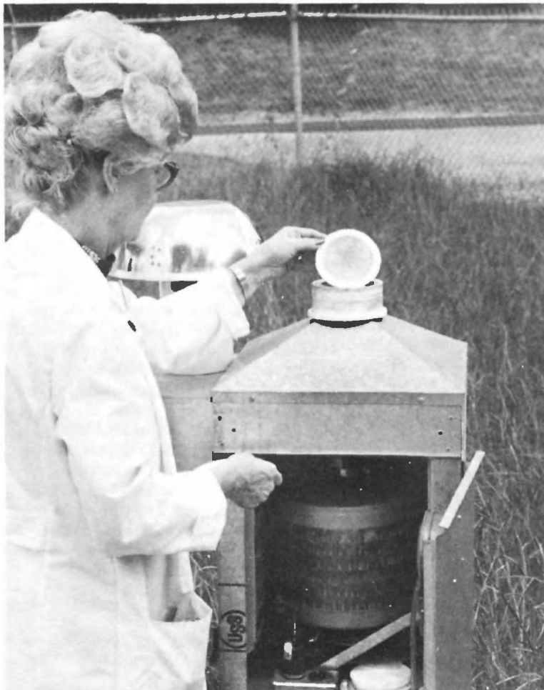
ERAMS air stations operator changing filters in air sampling unit. Filters are changed twice weekly.
