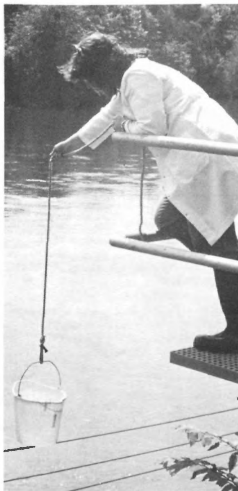
Collecting a surface water sample adjacent to the Montgomery, Ala., water treatment plant. Such samples are collected quarterly at ERAMS surface water sampling stations.
