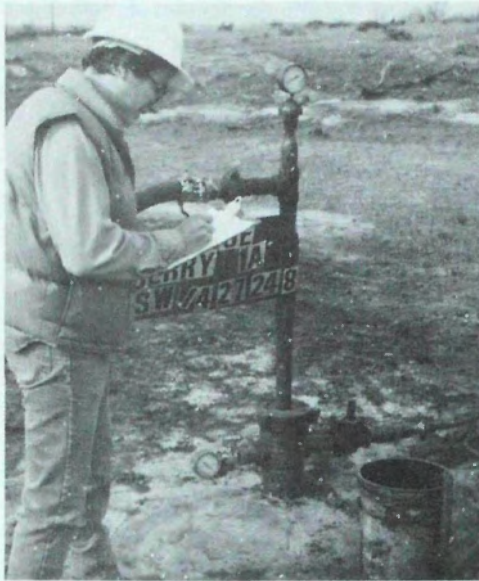
On Osage Indian lands in Pawhuska, OK, geological technician Andrew Yates records information from pressure test of injection well. Recent amendments to the Safe Drinking Water Act state that EPA may now deal with Indian tribes as sovereign entities in drinking water and ground-water matters
