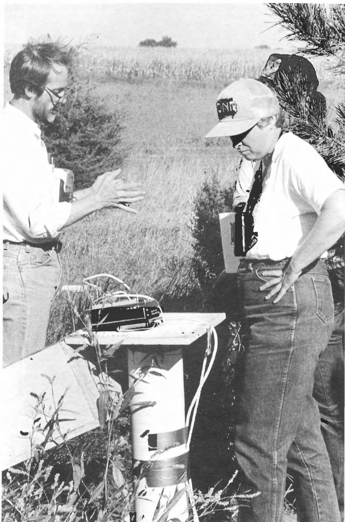
As part of Iowa's Big Spring Basin Demonstration Project, ground water is continuously monitored at more than 50 sites including this deep-monitoring well in Clayton County.
