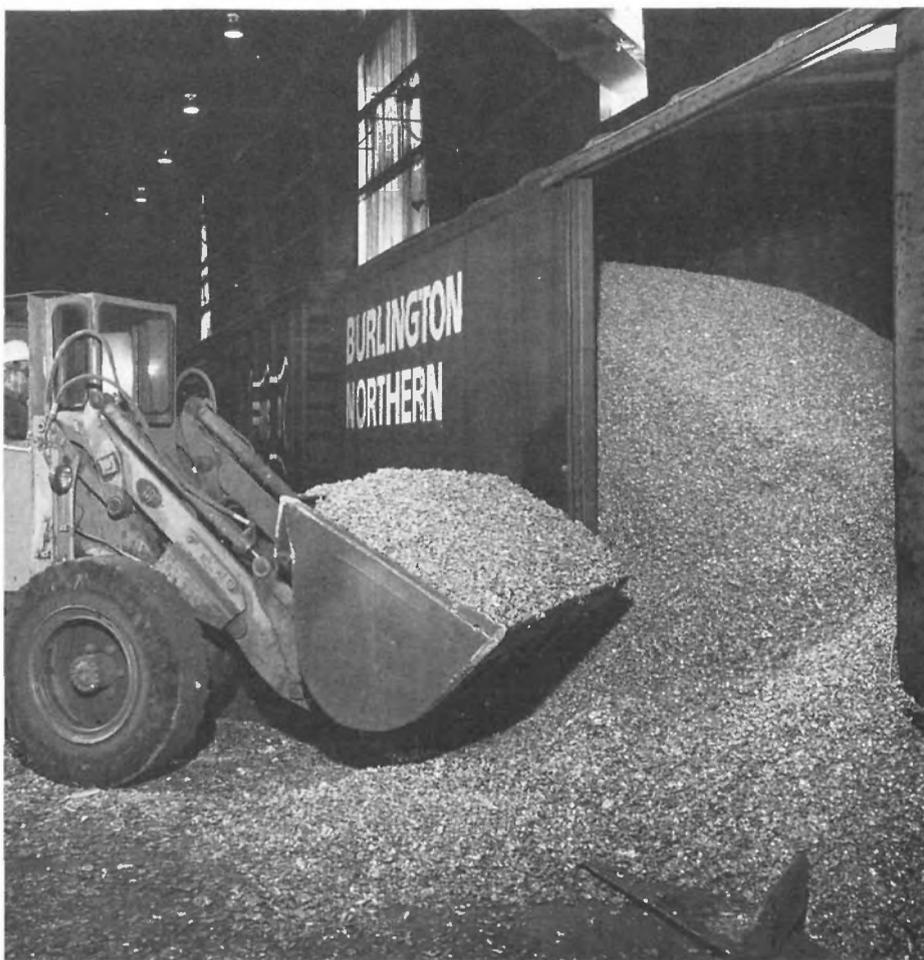
*Markets for scrap aluminum are strong. Here shredded aluminum cans arrive by rail at a Reynolds Aluminum reclamation plant. The cans will be off-loaded and fed into a furnace for melting.*
