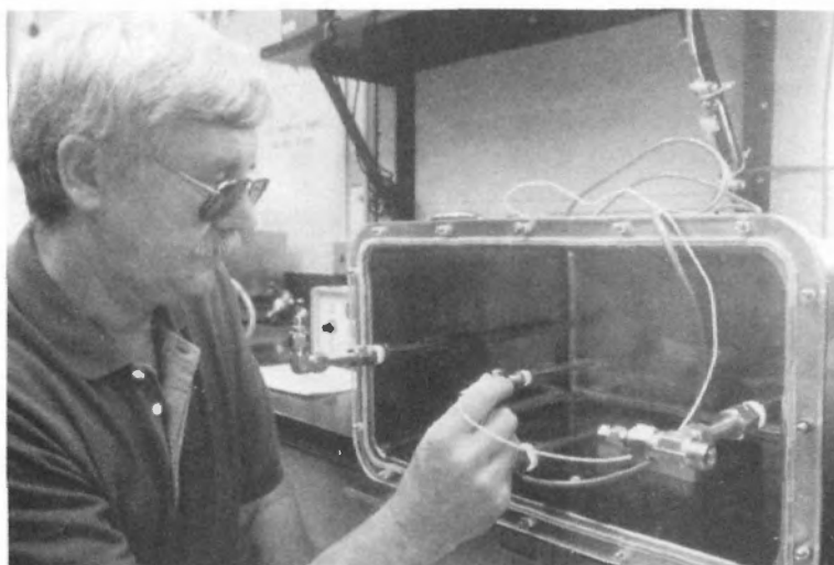
Bruce Tichenor, environmental engineer at EPA's Air and Energy Research Laboratory in RTP, North Carolina, adjusts a temperature probe for a small environmental test chamber. The interactions of so many factors (including temperature) make sick building syndrome difficult to study.
