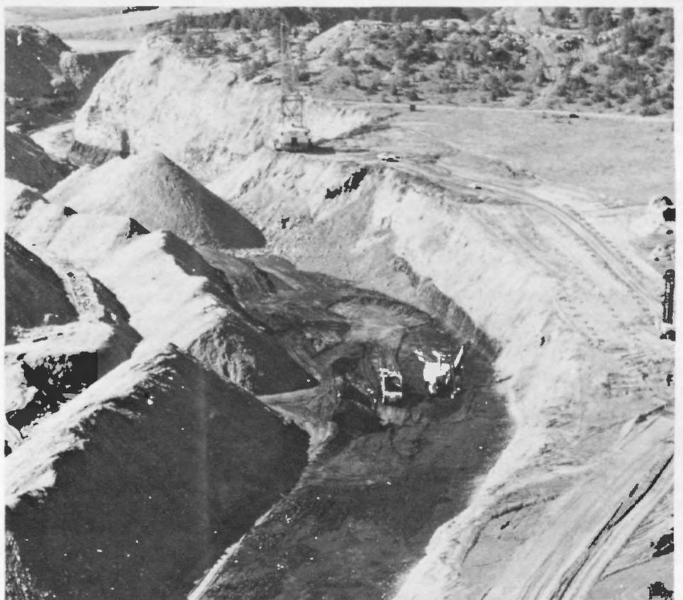
Hawk's eye view of the Montana strip mine shows wide, flat seam of black coal which is being dug by heavy machinery and hauled away by trucks.
