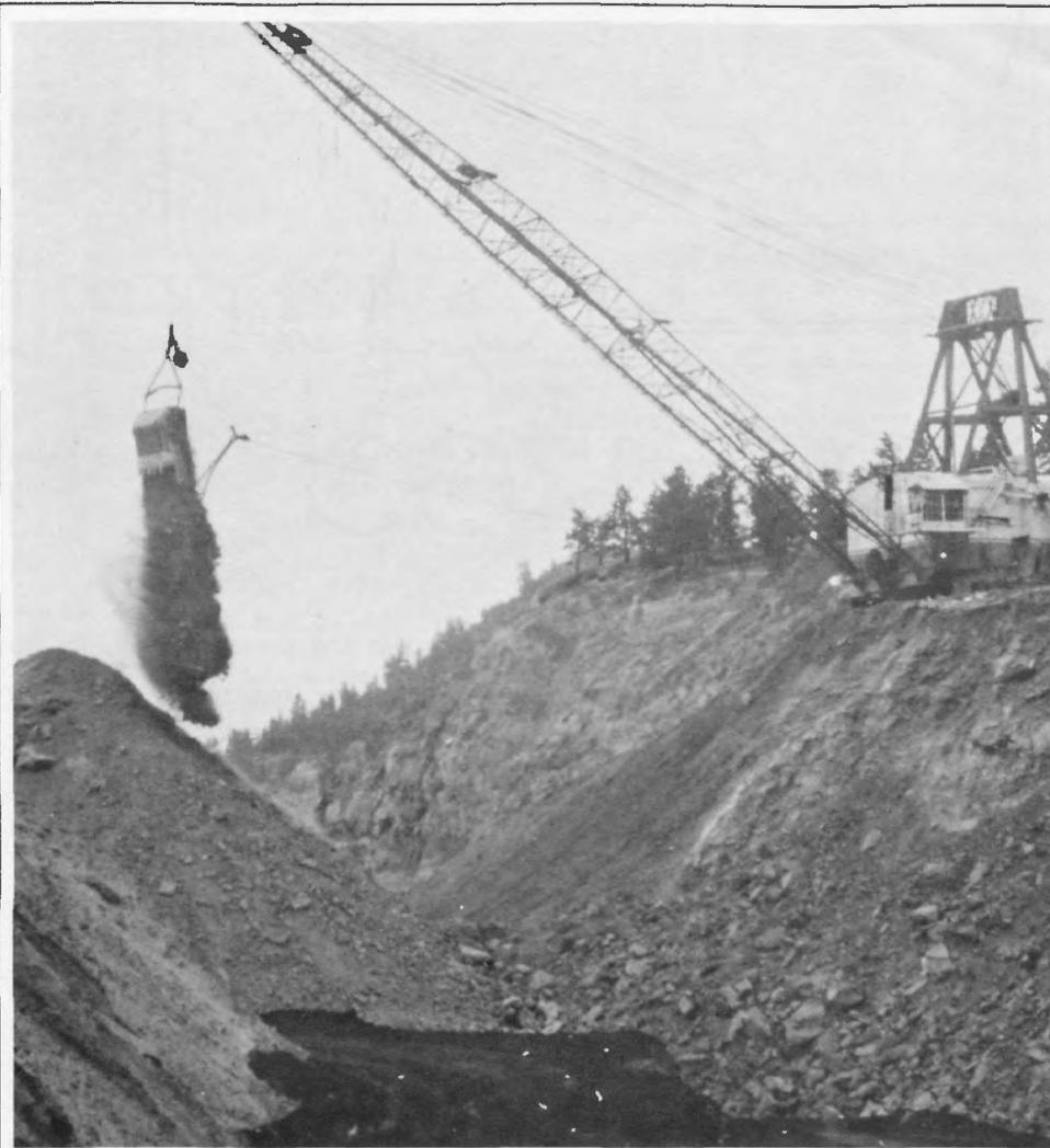
Dragline bucket scoops earth and rock "overburden" to expose the coal. New stripmined land in Colstrip area will be restored to meet Montana's exacting standards after the coal has been dug.
