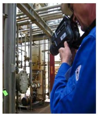
EPA inspector using an infrared camera to detect invisible organic chemical emissions. Photo: EPA.
